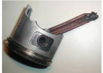
Fig 2:Actually Broken Connecting Rod Of The Bike
