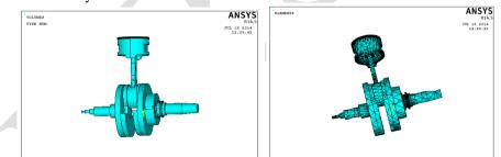
Fig 12: Imported model in ANSYS and Mesh Model for Carbon Fiber Connecting Rod in Assembly
