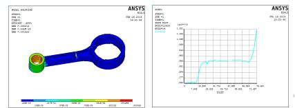
Fig 5: Strain induced .001426 On The Connecting Rod Of Al2014 and Starin On Connecting Rod Of Al2014
