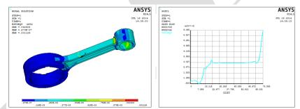
Fig 7:Strain induced .001129 On The Connecting Rod Of Al7075 and Starin On Connecting Rod Of Al7075
