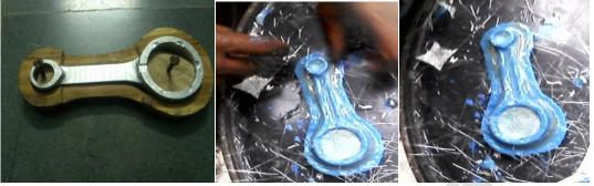
Fig 22: Mold Preparation
