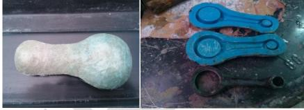
Fig 23: Fiber Glass Mold Preparation
