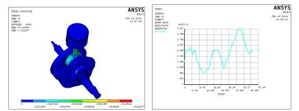
Fig 14: Strain on Carbon Fiber Rod In Assembly
