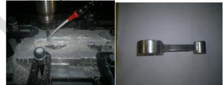
Fig 21: CNC machining of aluminum block
