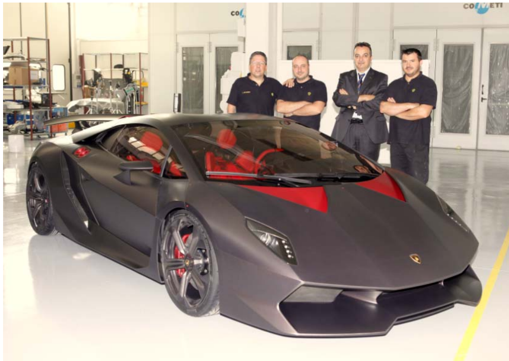
Figure 1. The 2010 Lamborghini Sesto Elemento , carbon fiber composite technology demonstrator.
