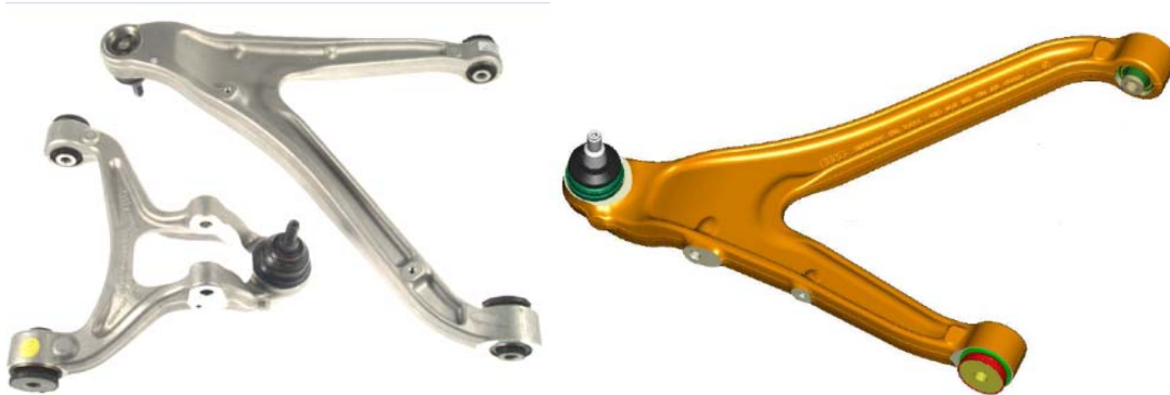
Figure 3. Front upper and lower aluminum arms (left) and CAD detail of front lower arm (right).
