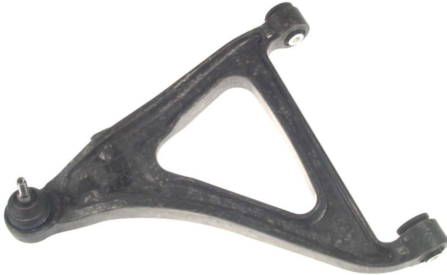
Figure 12. Front lower control arm after machining and installation of the bushings and ball joint.
