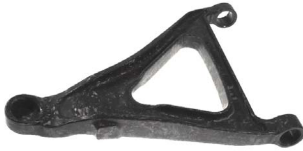
Figure 11. Two views of the as-molded front lower control arm.
