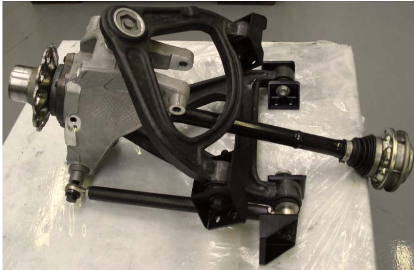
Figure 14. Rea upper and lower cotrol arms installed on the wheel assembly.
