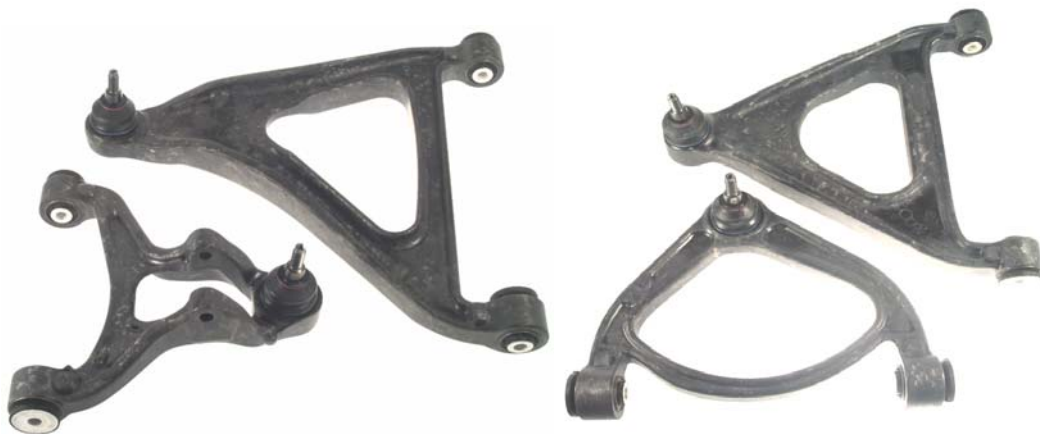
Figure 13. Front upper and lower arms (left), and rear upper and lower (right) control arms.
